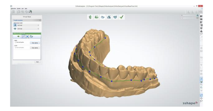
Next, build a horseshoe arch base for the model. As clear aligners are usually cut to the gingival margin of the patient's dentition, it is recommended to extend the base below the lowest point on the gingival margin by about 2 mm.
