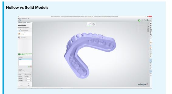
Hollowing the model can improve print time and reduce unit cost, although this feature is only available in certain orthodontic CAD softwares. If hollowing a part, ensure that wall thickness is at least 2-3 mm thick. Formlabs recommends printing solid models to reduce post-processing difficulty.
