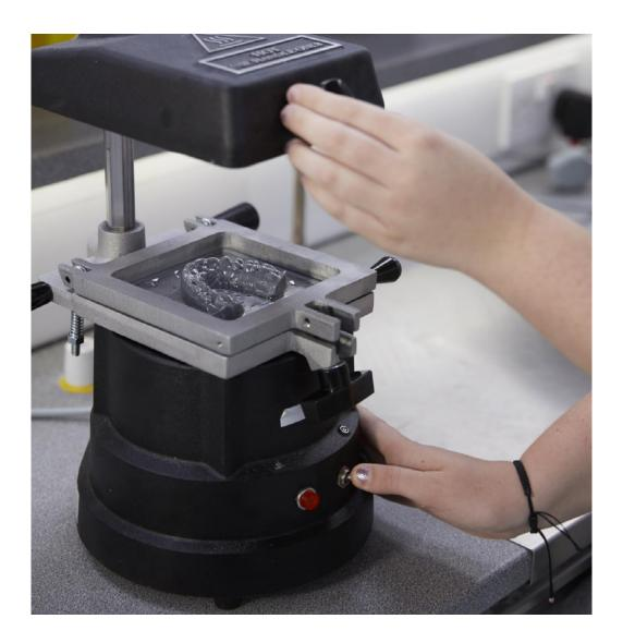
**Warning!** Depending on the aligner material being used, if the model base is too tall, the resultant aligner walls will be too thin. Ensure that the models generated are short enough for the recommendations provided by the manufacturer. Generally the recommendation is to keep model height below 19 mm.
