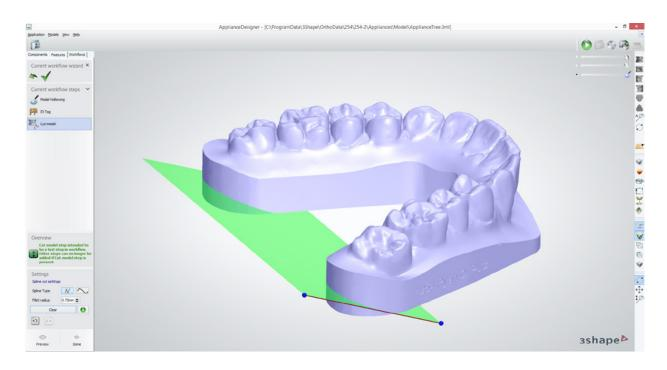
Chamfering the model base makes removing parts significantly easier. This can be done easily at the rear of the model with a plane cut tool.
